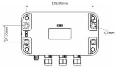
**3**: Mount the unit at a suitable place on the wall by inserting the screws through the holes provided in the housing and fastening the screws.
