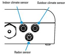
In case of a Radon sensor error, the display shows "Sensor error". The climate control system then continues to ventilate at the set interval.
