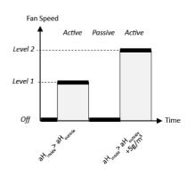
**Definition of the speed:** The speed is defined at the beginning of an active phase and is maintained during this phase. Therefore, the speed is only adjusted again with a new active phase.
