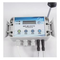
**5**: Connect the power cable as well as the actuators by passing the cables through the gland and connecting them to the appropriate terminals. The terminal blocks can be removed for this purpose.
