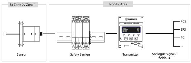
Typical system design for installation in Ex-Area
